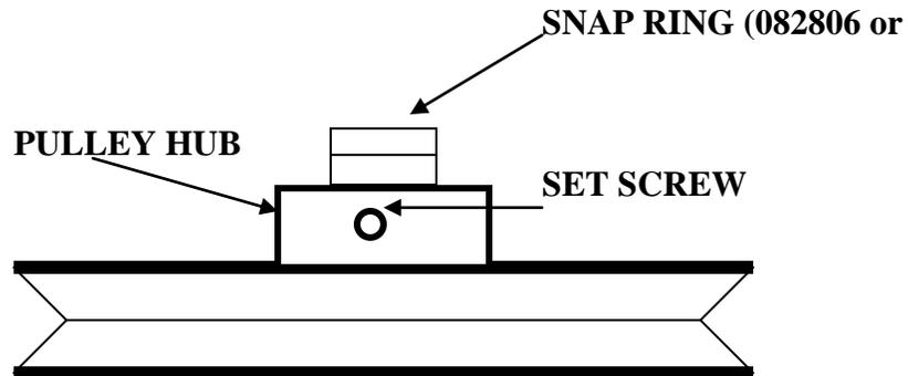
**NOTE; Units with serial numbers 082806XXX or later will have a snap ring securing the pulley to the shaft instead of the setscrew.**
