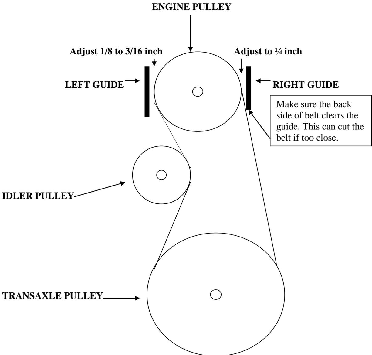
**This illustration shows the proper configuration of the drive pulley on the transaxle.**
